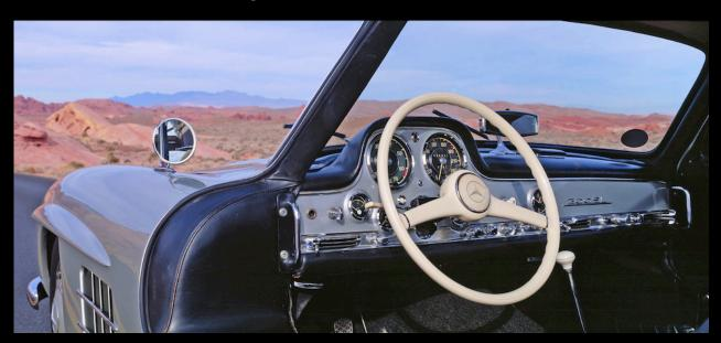
"Launched in 1954 at the New York Auto Show, the vehicle was aimed at the booming post-War American vehicle market and loosely based on the 1952 sports car of the same name. To save weight, the racecar laid a metal skin over a tubular metal skeleton, necessitating the gull-wing style doors, which were carried over to the customer model.
